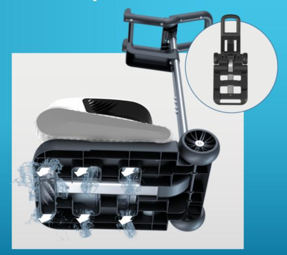
Robot water drainage is facilitated by the base and bottom brackets.
